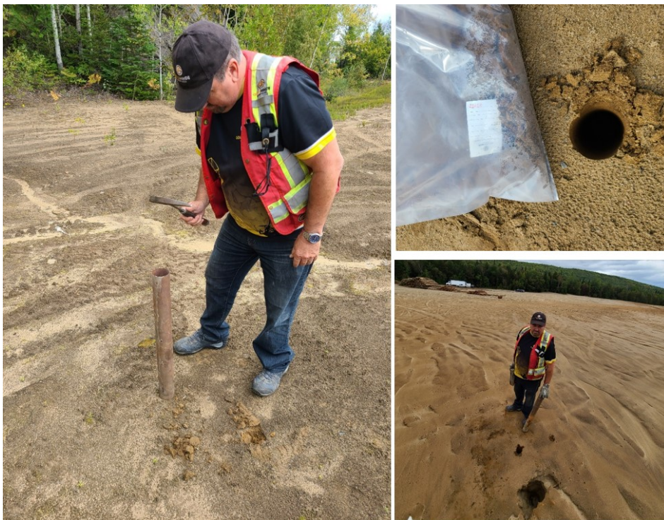
Figure 12.4: Surface sample collection from the Montauban tailings sites
